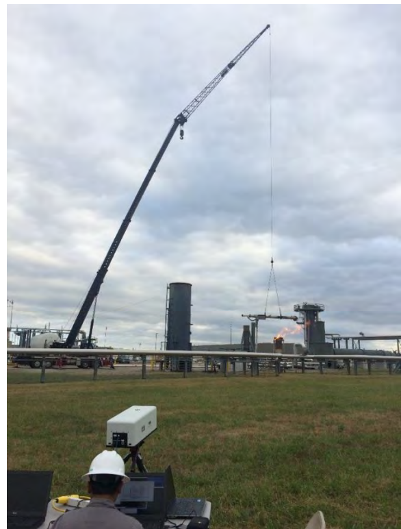
Figure 15. VISR method demonstrated as part of the PERF remote flare monitoring blind testing.
