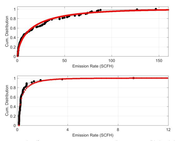
Figure 6: Top panel: Malfunctioning intermittent pneumatic controller emission rates (black circles) with fitted CDF (red line). Bottom panel: Properly functioning intermittent pneumatic controller emission rates (black circles) with fitted CDF (red line) excluding minimally emitting data.
