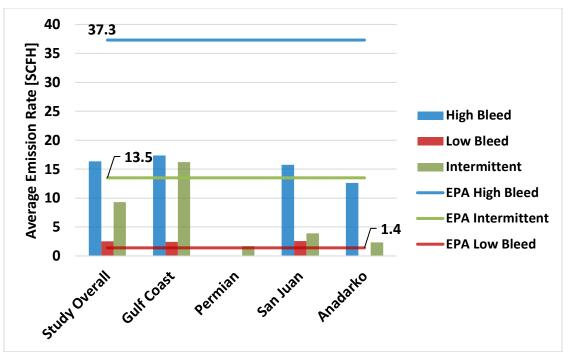
Figure 4: Average emission rates per controller by type and basin compared to US EPA Subpart W emission factors.
