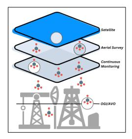
Figure 1. Multi-layered Approach for Leak Detection
