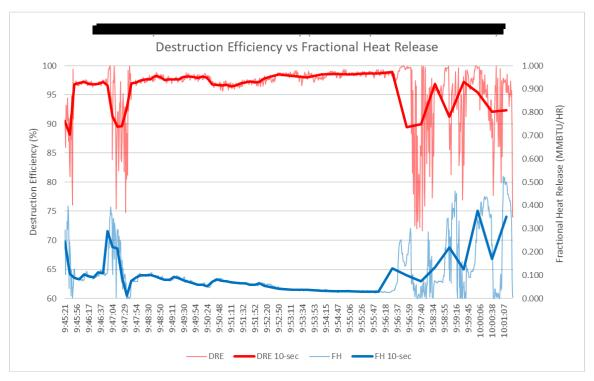
Figure 5: Destruction Efficiency vs. Fractional Heat Release and Smoke Index for
