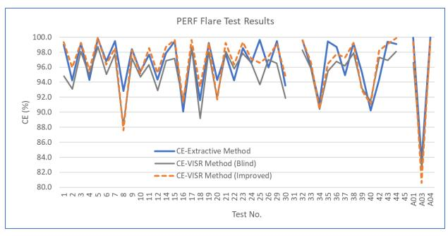
Figure 16. PERF test results, VISR (remote) vs. Extractive.
