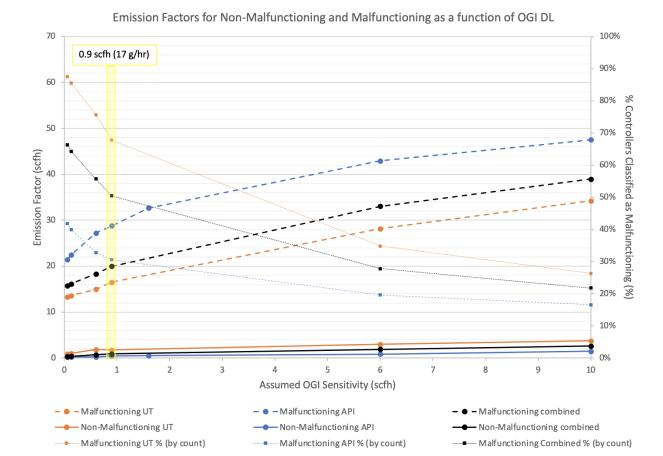
The assumed detection threshold exceeds 10 scfh before the non-malfunctioning (properly operating) average emission reaches 2.82 scfh (proposed factor).
