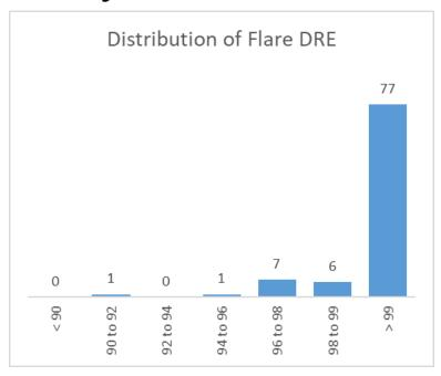
Figure 2: Distribution of Flare DRE measurements.
